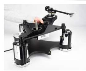
Gently install the subchassis onto the main chassis, ensuring that the subchassis legs are placed into the suspension adjusters positioned in the middle of each of the springs.
