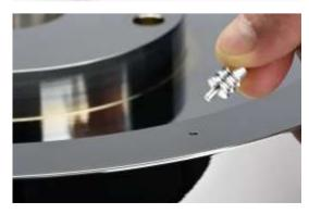
To install the drive belts, you must first attach them to the platter using the designated belt fitting pin.
